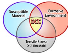
Figure 1 Schematic diagram showing the three factors on SCC of metallic materials.
